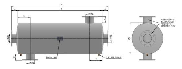
The ECI Residential Silencer is a high performance reactive silencer, recommended for those conditions where the ambient noise level in the environment is low. For use with two and four cycle diesel engines.
