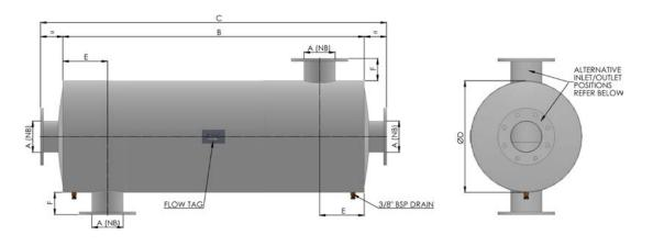
The ECI Industrial series of silencers are medium degree reactive silencers for use in environments where background noise is relatively high. Can be used with two and four cycle diesel engines.
